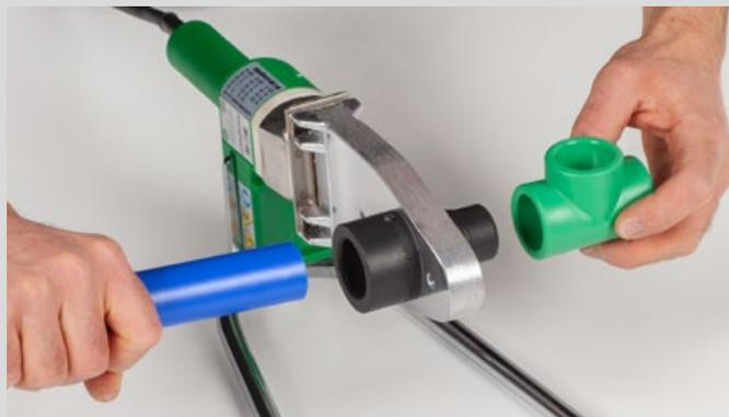
Heating-up of pipe and fitting
