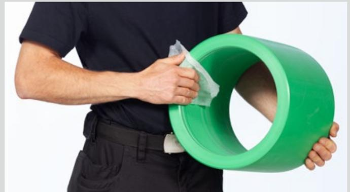
Clean the electrofusion socket's inner surface with a lint-free cloth or paper. Remove moisture that may occur **immediately before the welding process** again.
