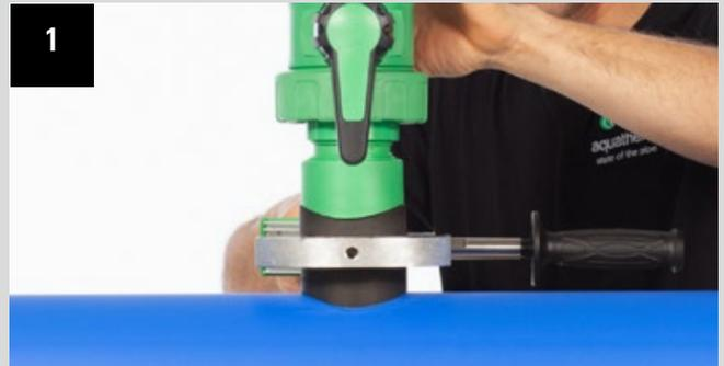
1. Welding-on of weld-on saddle set onto the main pipe
