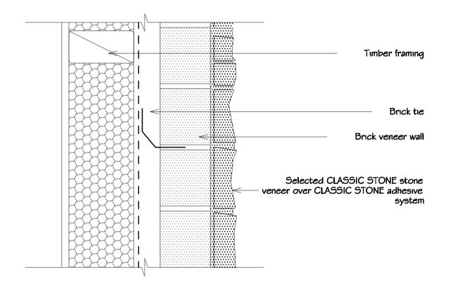
13 - Typical Stone Veneer over Brickwork
