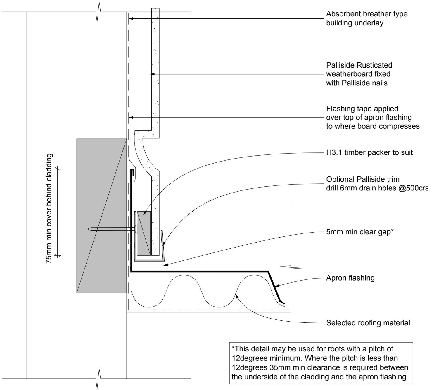
\*This detail may be used for roofs with a pitch of 12degrees minimum. Where the pitch is less than 12degrees 35mm min clearance is required between the underside of the cladding and the apron flashing
