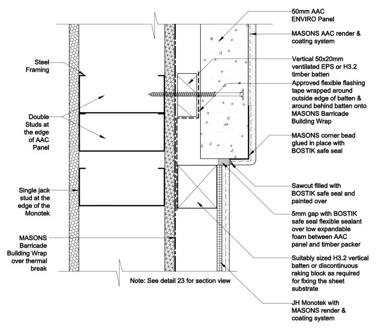
**OPENING FLASHINGS ENVIRO AAC PANEL / MONOTEK Vertical Junction for above Windows** & Doors
