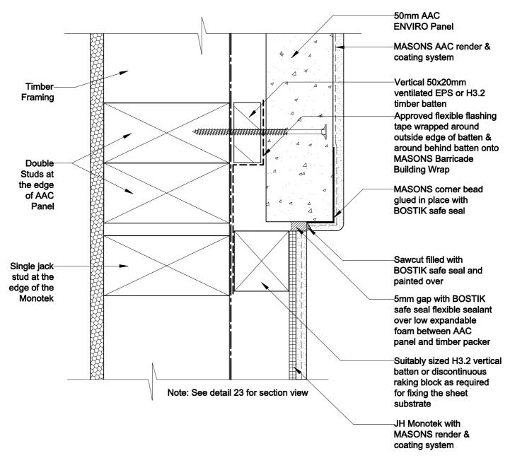
**OPENING FLASHINGS ENVIRO AAC PANEL / MONOTEK Vertical Junction for above Windows** & Doors
