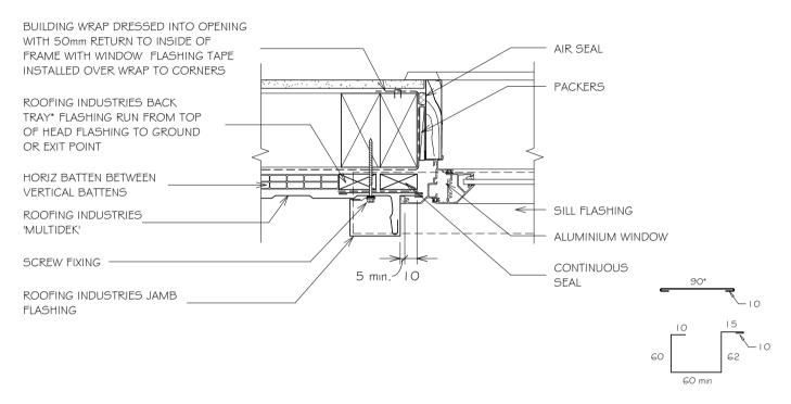
\* Back tray size may require to increase to ensure coverage at ends of head flashling. (Dimensions are indicative only) Turn down end of head flashing
