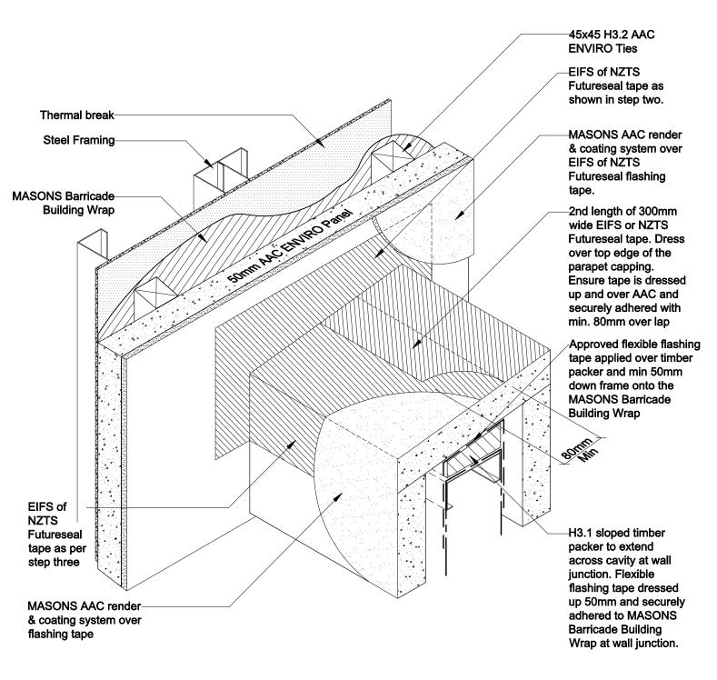
PARAPET / HANDRAIL TO WALL JUNCTION ENVIRO Panel Capping Step 4 **Detail 59C NTS**
