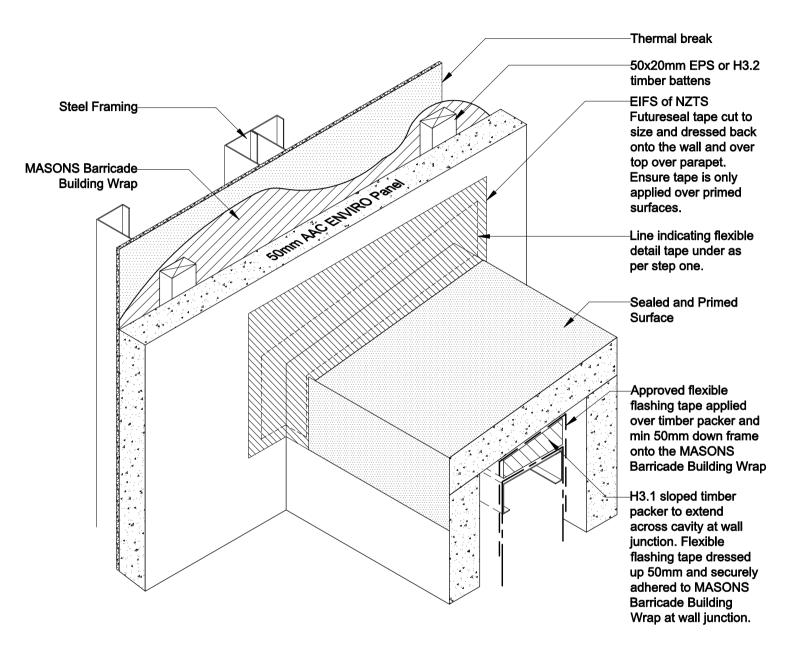
PARAPET / HANDRAIL TO WALL JUNCTION ENVIRO Panel Capping Step 2 **Detail 56A NTS**
