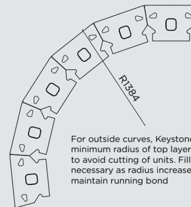
For outside curves, Keystone Compac® S minimum radius of top layer shall be 1400mm to avoid cutting of units. Fill pieces will be necessary as radius increases in lower units to maintain running bond
