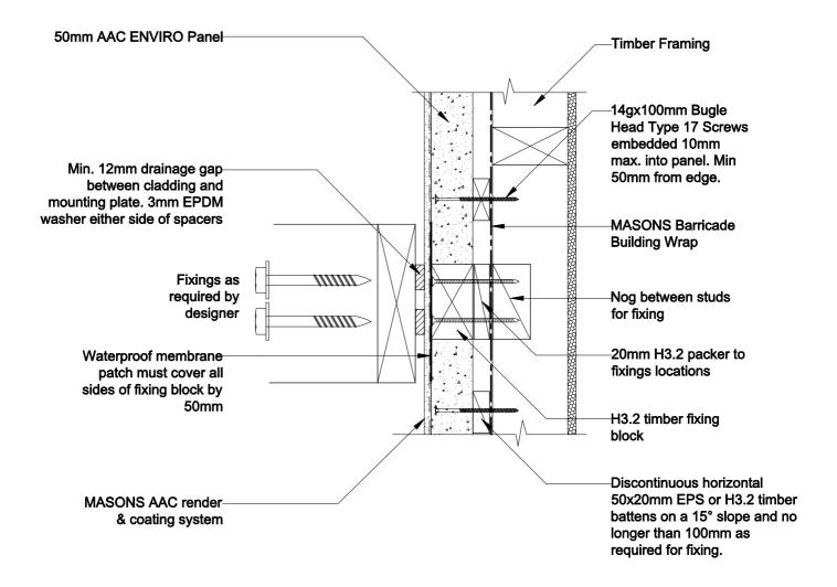
**DECK / PERGOLA EXTERIOR Wall Fixing**  Detail 36 Scale 1:5 Note: Detail to be drawn to specific design
