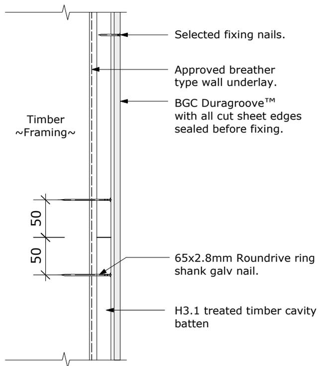
PROFILE **BGC Duragroove™**DATE **Nov 2011**DETAIL **Joining of Structural Batten**SCALE **1:5 @ A4**DETAIL NO. **D 15**
