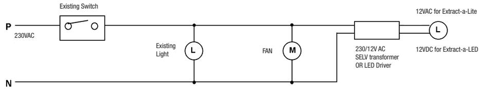
**Diagram 2 (EL100T) Timer Model. This diagram is for a lighting circuit only**
