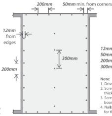
12mm min. from edge 50mm min. from corner 200mm centres max. at sheet perimeter
