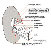
Left & right hand kick-out flashings are available. One piece stop end flashing.
