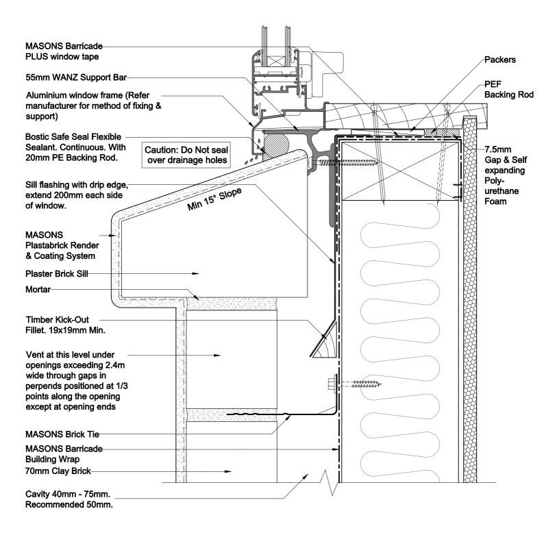
**OPENING FLASHINGS**Window Sill - Brick
