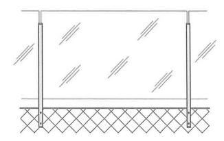
10mm Glass, Inline - Semi Frameless, Top Mount or Face Fix (Glass edge flush)
