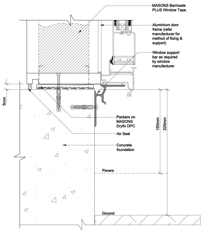
OPENING FLASHING CONCRETE DOOR SILL
