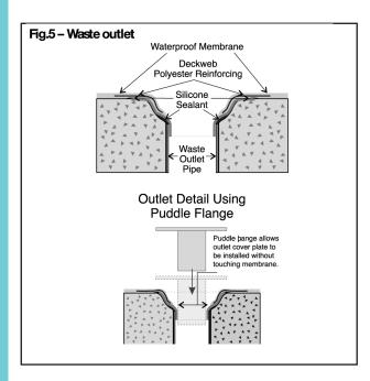
the edge of flange by at least 30mm. Place ARDEX "Deckweb" polyester woven mat reinforcement over the applied membrane. Thoroughly wet out the cloth and remove all creases in, or air pockets under the mat. Immediately apply a second coat to completely fill the mat. (Refer Fig. 5)
