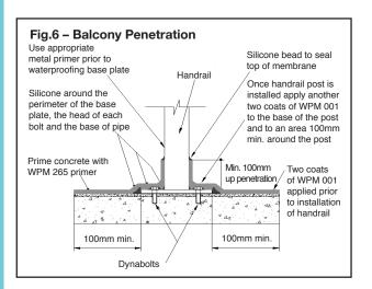
perimeter of the penetration. Apply the first coat of ARDEX WPM 001 on the substrate and the flanged metal.
