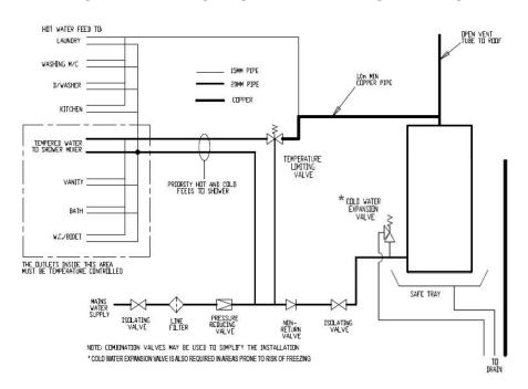
Marning: For closed (valve vented) installations a pressure relief valve must be fitted in the installation. Relief valve rating 7 kW minimum. Refer main label for pressure rating. The valve or drain valve outlet pipe must not be sealed or blocked. The first metre of drain line from the relief valve must be in copper.
