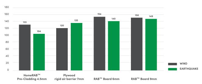
Bracing units per metre (length 1200mm)
