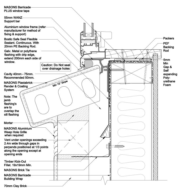
**OPENING FLASHINGS Window Sill - Aluminium**
