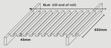
DescriptionSizeMasons CodeInsul-Baffle separator - 2 pack box45mm x 650mm x 6LmBFFL.5X650x6
