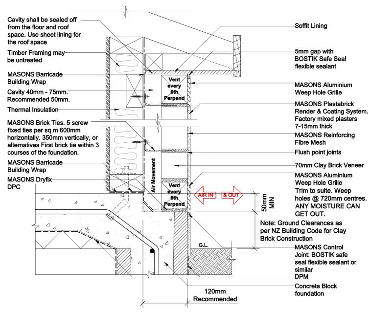
"70 series clay brick installed and plastered per MASONS Plastabrick Manual - 2014. Final colour and texture to be selected"
