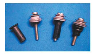
When fibreglass sheeting is lapped onto metal sheeting a T17 coarse treaded self drilling screw with a 32mm Weatherlok Seal fastened into the top of the rib, provides a firm seal in the lapping joint. The table below indicates the recommended spacing for side stitching fasteners.
