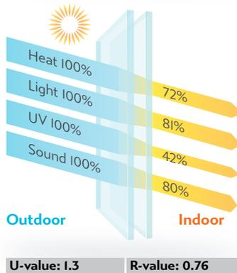
\* The use of tinted or reflective glass leads to higher absorption of solar radiant heat, this results in higher thermal stress which may lead to fracturing of the glass pane. Heat strengthened or toughened glass may be required. Talk to your Fairview fabricator for more information.
