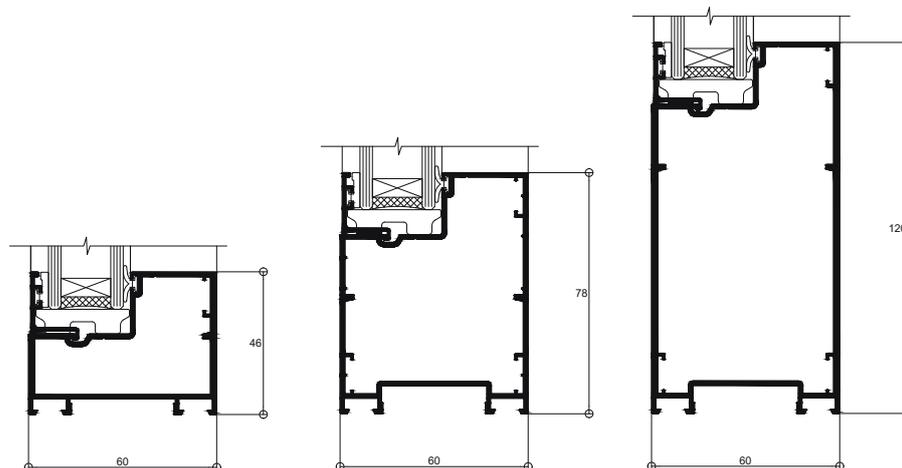
\* A manufacturing technique called "tipping" allows larger stiles to be used with smaller rails.
