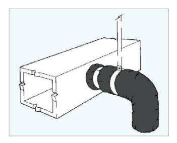
Support the duct between a metal connection and bend by allowing the duct to extend straight for 100mm before making the bend.
