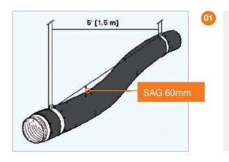
Flexible duct shall be supported at intervals, no greater distance than 1.5m. Maximum permissible sag is 40mm per metre of spacing between supports.
