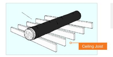
Flexible ducts may rest on ceiling joists or truss supports. Maximum spacing between supports shall not exceed 1.5m.
