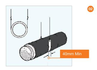
Hanger or saddle material in contact with the flexible duct shall be of sufficient width to prevent any restriction of the internal diameter of the duct when the weight of the supported section rests on the hanger or saddle material.
