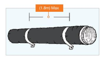
Vertically installed duct shall be stabilised by support straps at a max of 1.8m.
