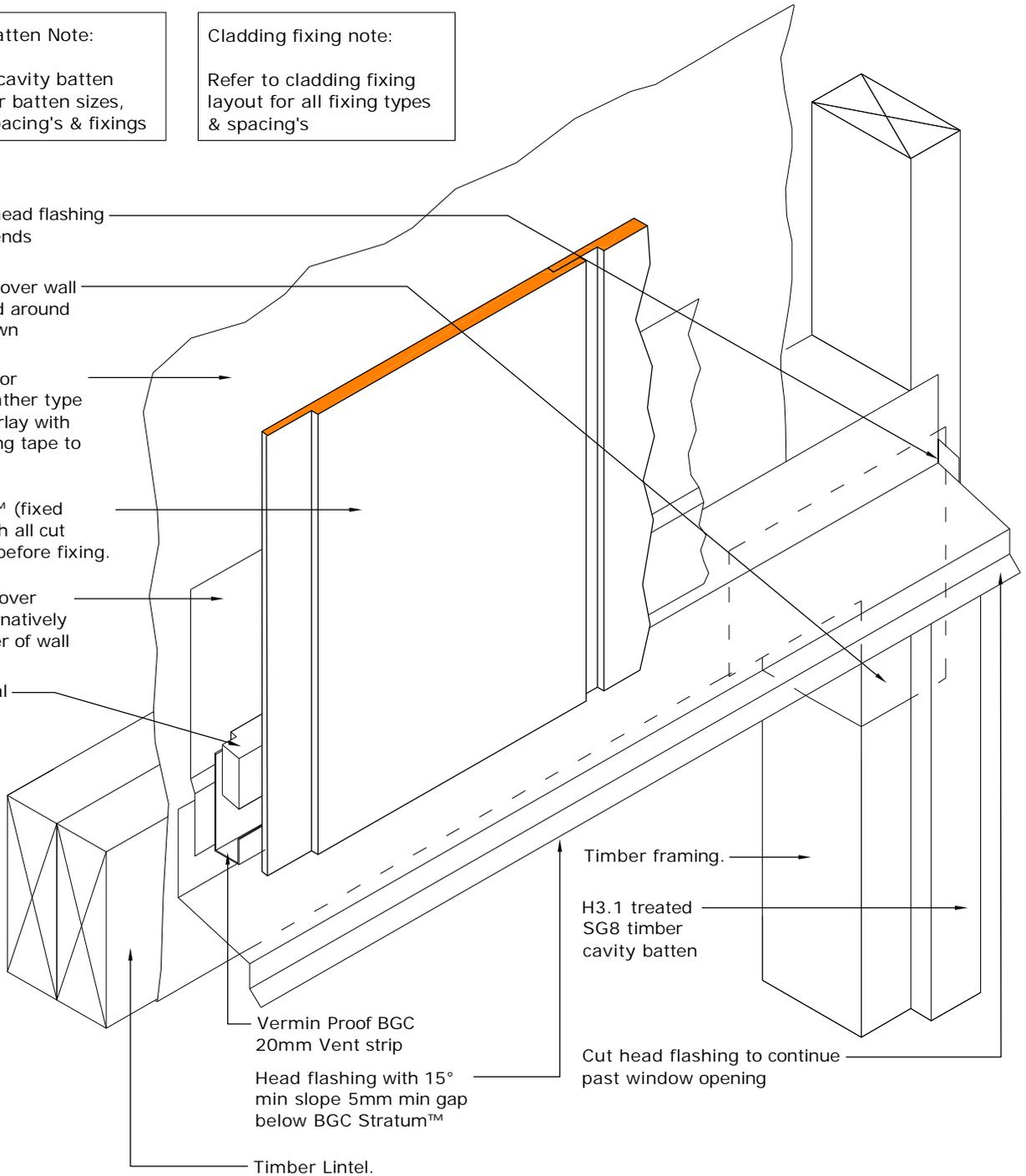
Note where Durabarrier™ is used flashing tape must be applied to the entire opening
