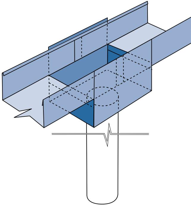
Internal sumps must have overflows. These are often a secondary pipe overflow with the outlet height positioned above the level of the primary outlet.
