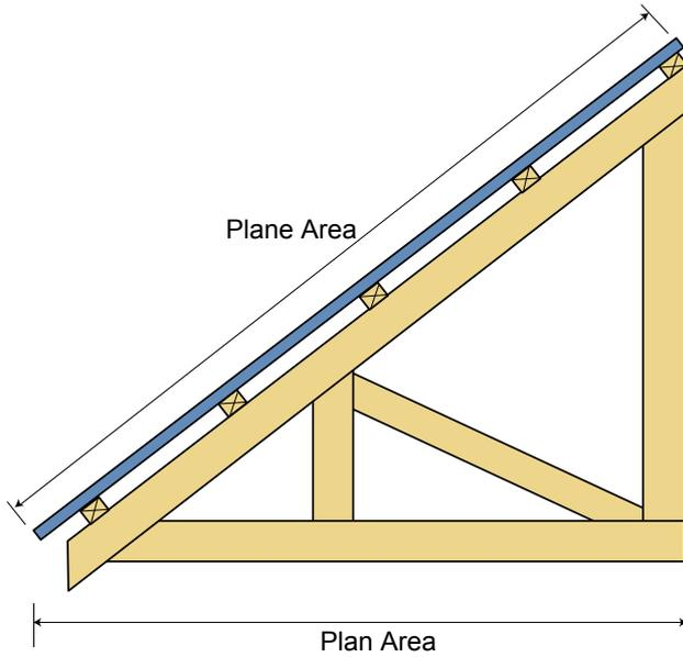
Wind action can influence effective catchment area, and the COP assumes the worst case scenario, i.e., rain striking the roof at an angle perpendicular to the roof plane.
