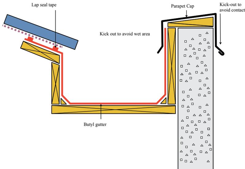
Suitable non-ferrous metals include 0.9 mm aluminium, 0.6 mm stainless steel, and 0.6 mm copper. Contact between coated metal products and copper or stainless steel must be avoided because it will lead to early corrosion. Splashback or runoff from copper onto coated metal can have the same effect.
