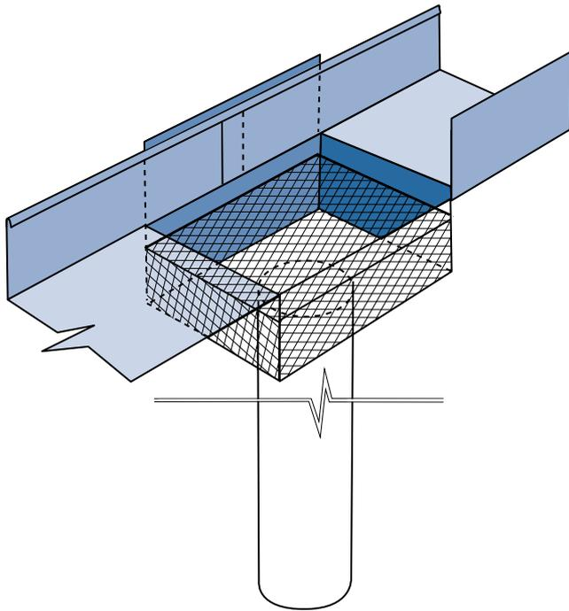
Gratings or guards should be designed so that any debris will float, and hail, or obstructions, such as a tennis ball, will not wedge and block the guard. Gratings or guards should be cleared of accumulated debris regularly as part of normal maintenance.
