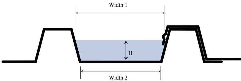
Effective cross section area of a trapezoidal profile is calculated by the width of the trough and depth to the bottom of the capillary groove
