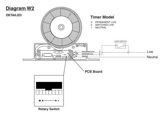
9. Remove the cover on the Fan Bracket and make the electrical connection as follows:
