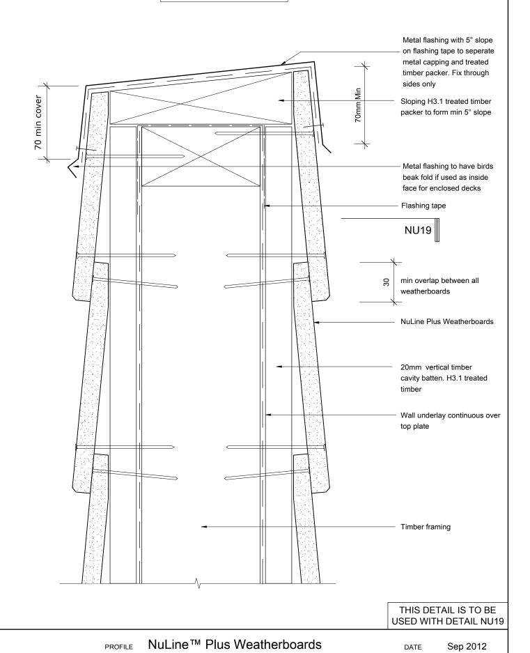
**Enclosed Balustrade/Parapet Wall**
