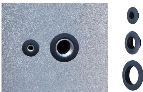
There are 14 plastic fitting surrounds, these vary in size and should fit tightly around the fittings. The fitting surrounds are placed on after the panel and should sit flush with the front of the fitting. Attach the fitting surrounds as each panel is put in place, this will help to hold the section in the correct position as each panel is added.
