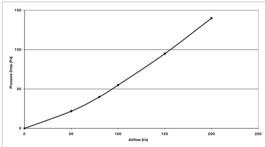
The resistance curve has been constructed from numerical and empirical measurements of the pressure drop across the filter for a range of in-line duct flow rates.
