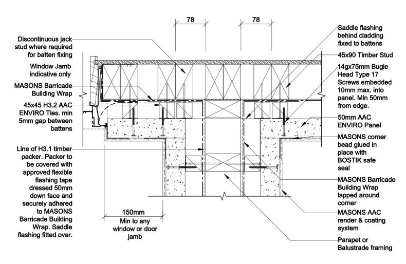
PARAPET / HANDRAIL TO WALL JUNCTION With Metal Capping Detail 44 Scale 1:5
