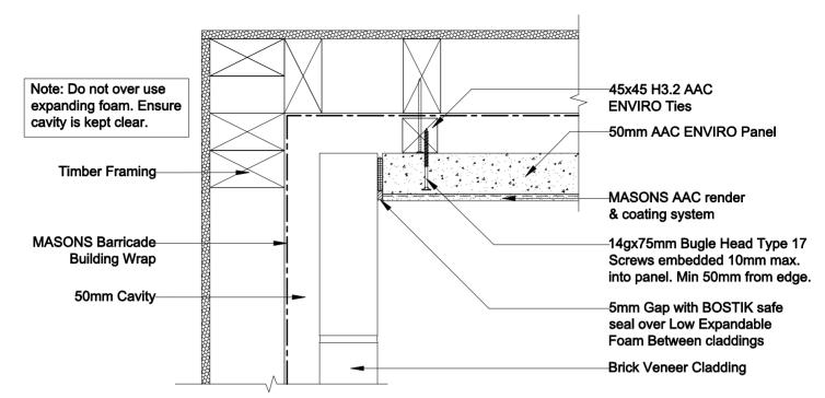
**AAC ENVIRO PANEL /** Detail 36 Scale 1:5 **BRICK VENEER - Internal Corner Junction** Timber Studs 45x45 H3.2 AAC **ENVIRO Tie** Brick veneer cladding with 50mm cavity MASONS Barricade **Building Wrap** 14gx75 Bugle Head Type 5mm Gap with 17 Screws embedded **BOSTIK Safe Seal** 10mm max. into panel. over Low Min 50mm from edge. **Expandable Foam** Between claddings Note: Do not over use expanding foam. Ensure 50mm AAC cavity is kept clear.
