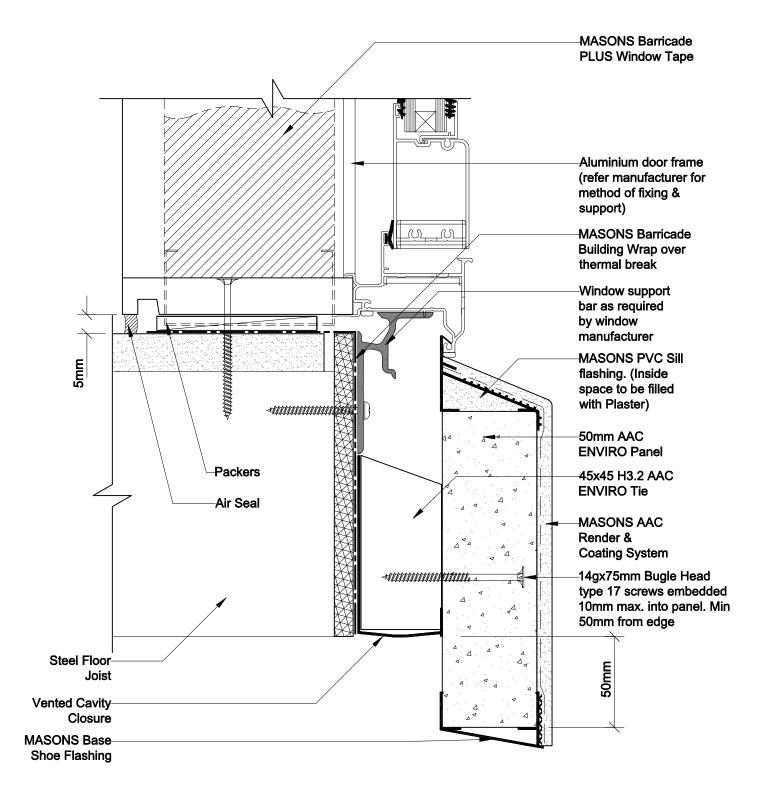
**OPENING FLASHING -**STEEL FLOOR DOOR Sill
