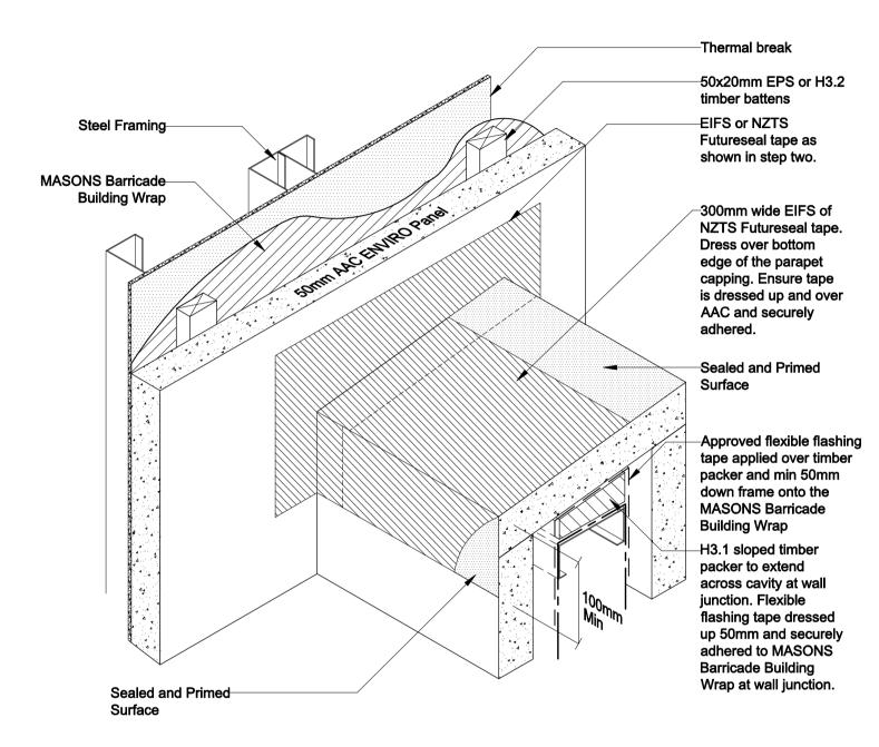
**PARAPET / HANDRAIL** TO WALL JUNCTION **ENVIRO Panel Capping** Step 3
