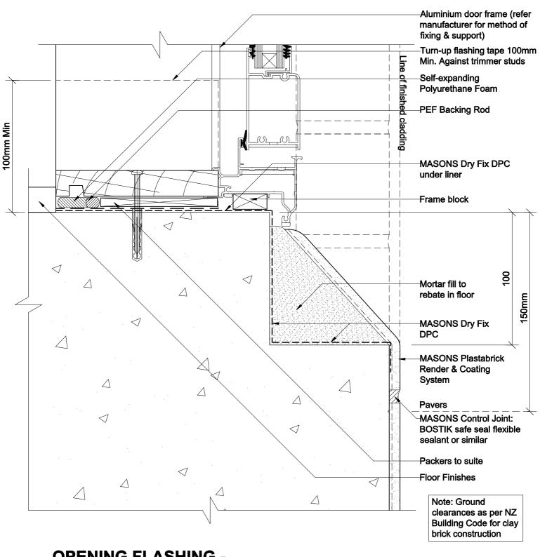
OPENING FLASHING - CONCRETE DOOR SILL With Rebate
