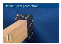
Making a windproof and weathertight joint to planed rafters or trusses with TESCON EXTORA. Taping sequence: 1st bottom, 2nd left and right hand sides, 3rd top.
