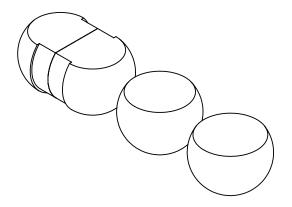
Internal operating volume Tank 1 3,243.6L Internal operating volume Tank 2 1,881.7L Internal operating volume Tank 3 1,809.5L
