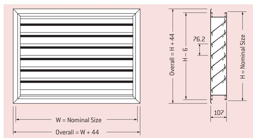
**Model: OHL 102 and OHL 124** are available in conventional unit construction, with a maximum blade length of 2.8 metres, or for greater lengths an architectural style is available to give continuous line, uninterrupted by mullions or surrounds. Louvers can be either pre-fabricated or pre-cut and supplied in sections for field erection on sites with more difficult access. Blades snap into concealed mullion clips.
