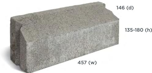
Firth Mountable Kerbs are used to form road edging and are ideal to form the edges of traffic islands and crossings. Mountable Kerbs have a sloping face rather than an abrupt angle and this enables vehicles to drive over them easily. Laid in the same way as Firth Road Kerbs.
