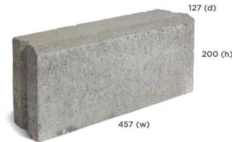
Firth Road Kerbs are designed to create the kerb on road network pavements. They can also be used to form the perimeter to car-parks and access ways. Firth Road Kerbs are laid in a concrete haunch with the V joint between units filled with mortar so they lock together.
