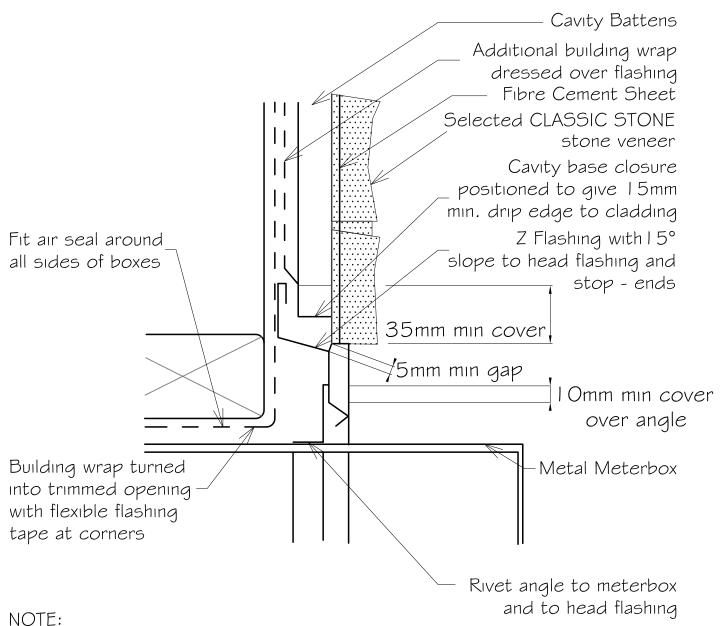
(1) Fix angle and seal to sides of box. At sides and base, *claddings* shall overlap angle by 10mm minimum. Continuously seal *cladding* against angle.
