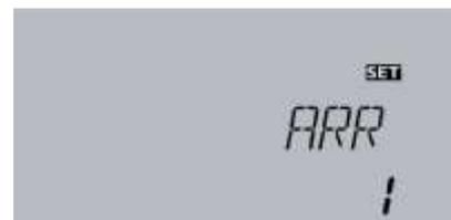
**Important note:** The subsequent selection of a different arrangement (at any stage during the operation of the controller) will reset all other adjustments to the factory settings, and thus all parameter settings will need to be verified and re-adjusted if required.
