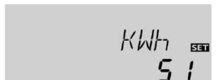
The flow rate as well as the values of the reference sensors S1 (flow) and S4 (return) are used for calculating the heat quantity supplied. It is shown in kWh in the channel **KWh** and in MWh in the channel **MWh**. The overall heat quantity results from the sum of both values.
