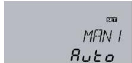
Note: Always adjust the operating mode back to “Auto” when the control and service work is completed. Otherwise normal operation will not be possible.
