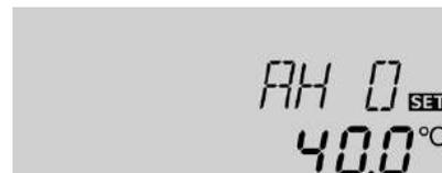
AHF: Thermostat switch off temperature.
