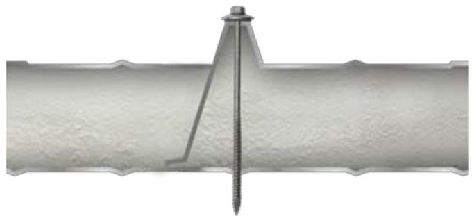
Composite panels are interlocked together.
