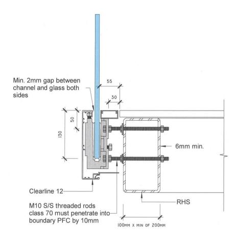
Steel members to be designed by Engineer CPEng. Spacing limited by glass capacity - refer to PS1 certificates
