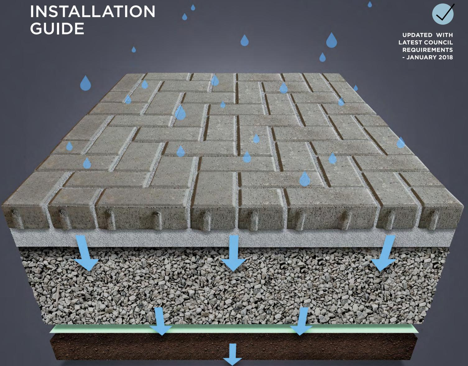
The Firth EcoPave® range will assist in the management of rain and stormwater runoff.
