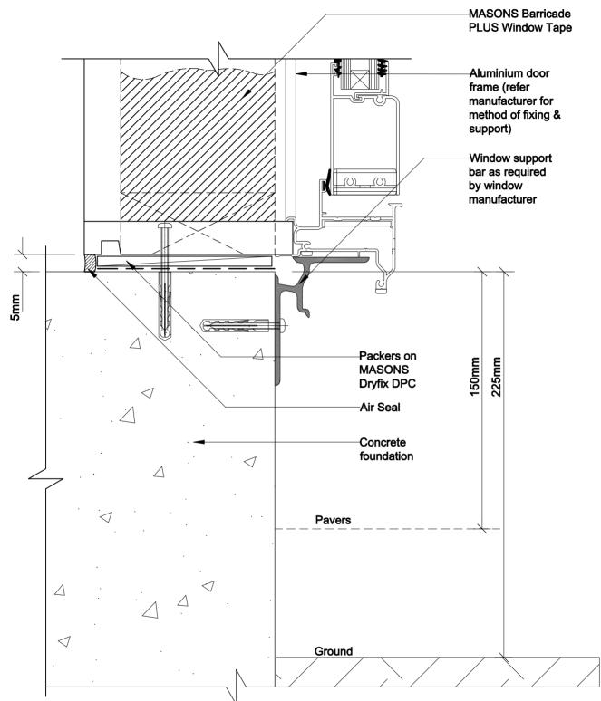
OPENING FLASHING CONCRETE DOOR SILL
