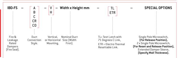
Fire and Leakage Rated Dampers shall be interlocking blade, curtain type, with stainless steel side seals conforming to AS 1530.4 - 2014 leakage requirements and having up to 4 Hour Fire rating.
