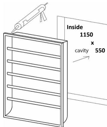
7. Prop back into position and allow to set for 24 hours minimum
