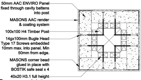
**AAC ENVIRO** cavity battens **COLUMN/POST - Plan View**
